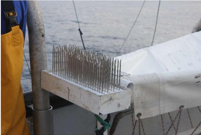
**Picture 8: Conventional tagging cradle with 100 tag block ready for tagging.**
