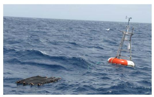
Figure 10. buoy at 5N, 155W with purse seine drifting FAD tied to it and a strobe light on the frame
