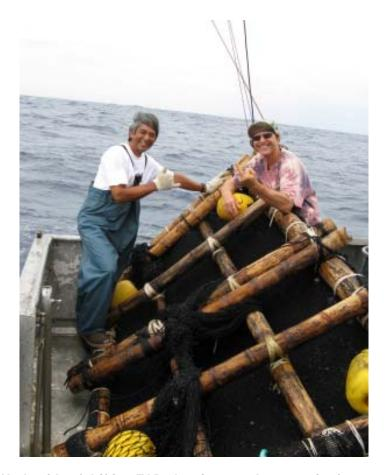
Figure 11. Underside of drifting FAD showing attachment point for 20 m aggregator
