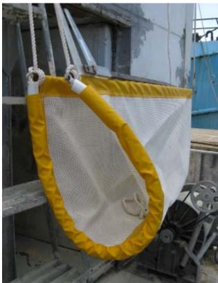
Figure 7. Lifting sling for large tuna
