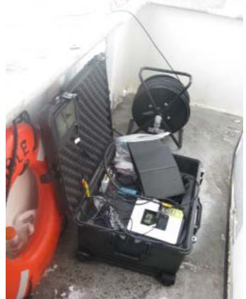
Figure 22. SPLASHCAM system showing video head, stabilizing fin and weight cabled to viewing and recording gear
