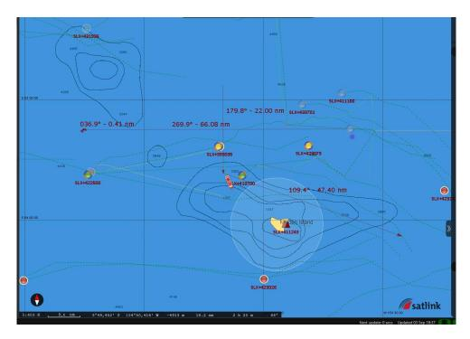
Picture 11. Array of 7 VR4-Global instrumented dFADs around Malden Island, Kiribati.
