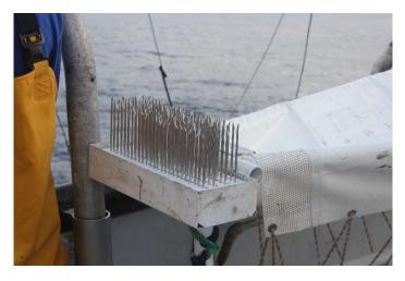
Picture 8: Conventional tagging cradle with 100 tag block ready for tagging.
