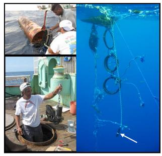
Figure 5. VR2 receiver mounting system.
