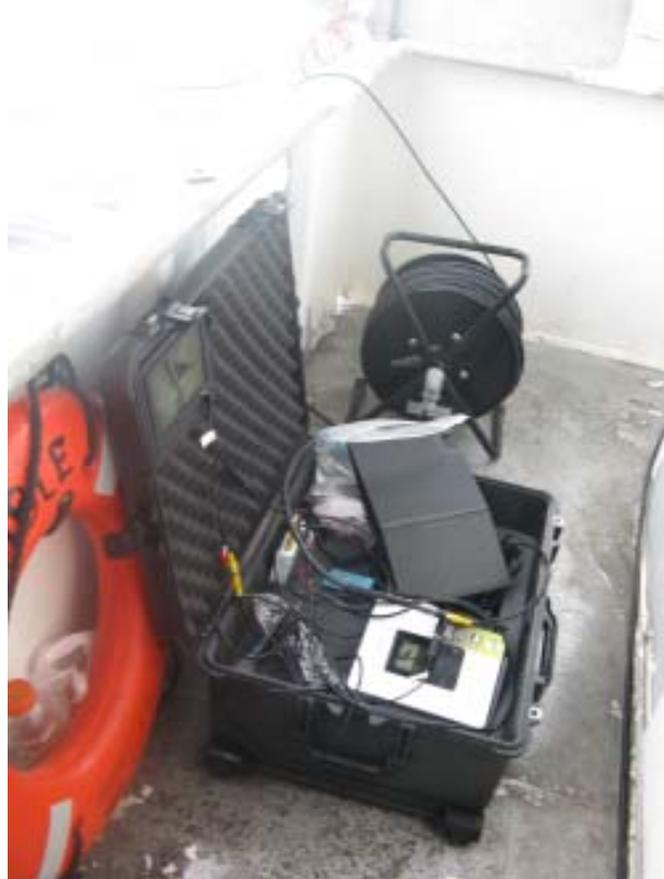
**Figure 22. SPLASHCAM system showing video head, stabilizing fin and weight cabled to viewing and recording gear**
