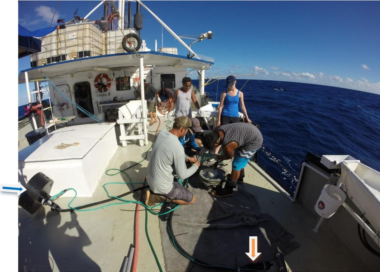
**Picture 5: Attaching a VR4 receiver to a dFAD. Blue arrow shows the unit and orange arrow the hydrophone**
