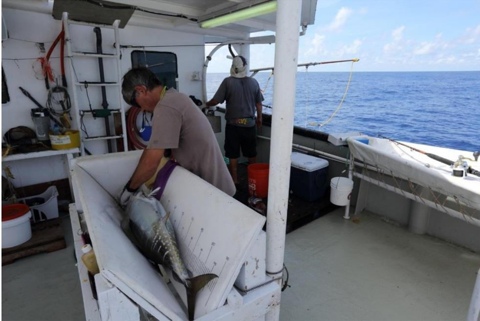
Picture 3: Archival tagging cradle (first plan, with a medium-sized bigeye ready to be tagged) and, at the back, 1 of the 3 conventional cradles.
