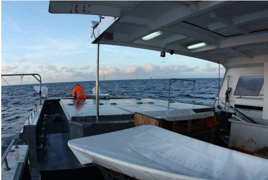
Picture 4: Deck set up showing the first conventional tagging cradle in the foreground, the archival cradle in front of fish holds and the second conventional tagging cradle at the stern.
